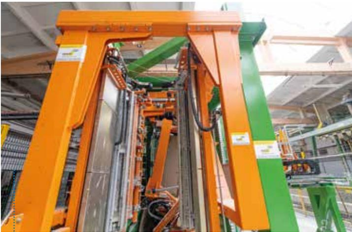
The cutting line with a tilting table to put an AAC cake upright the GSM.
