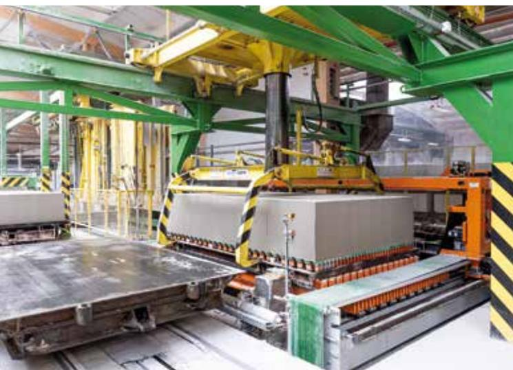
*The GSM moves a complete block raw to some millimetres to raise a gap between them.*
