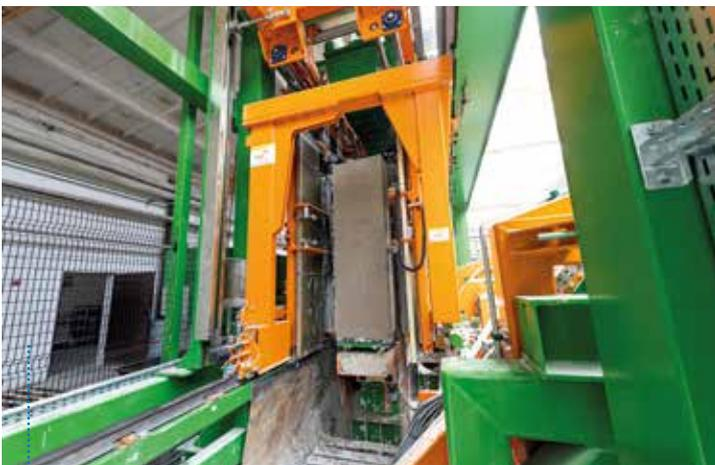
Two single wires cut a large variety of block sizes and formats.
