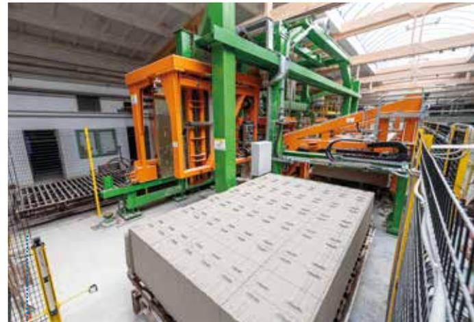
The retrofitted cutting area of the AAC plant.
