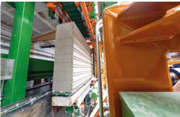
The tongue and groove system is inserted by the active horizontal cutter.
