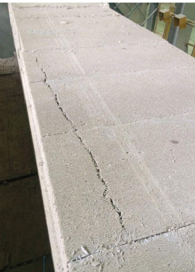
Fig. 2: AAC cake deformations
