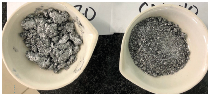
Fig. 3: Aluminium pastes partially agglomerated
