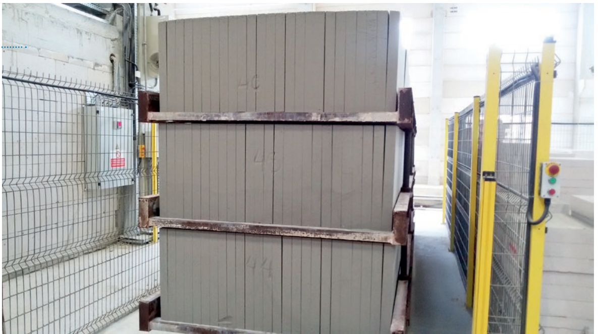
Separated Multipor insulation panels
