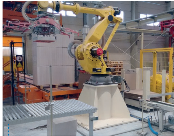
Packing line for Multipor insulation panels
