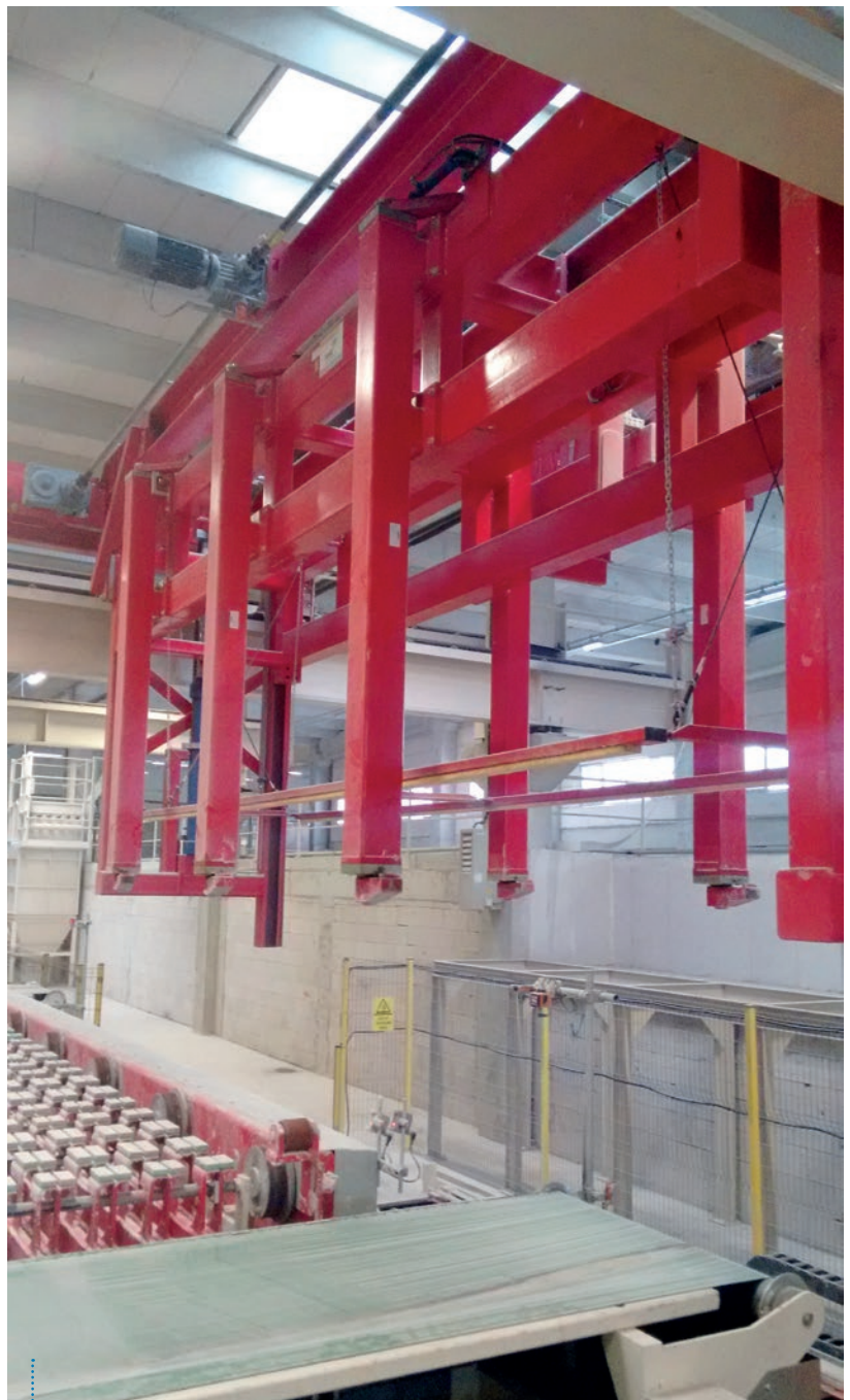
The manipulator is used to put an autoclave grate with the AAC cake onto the GSM
