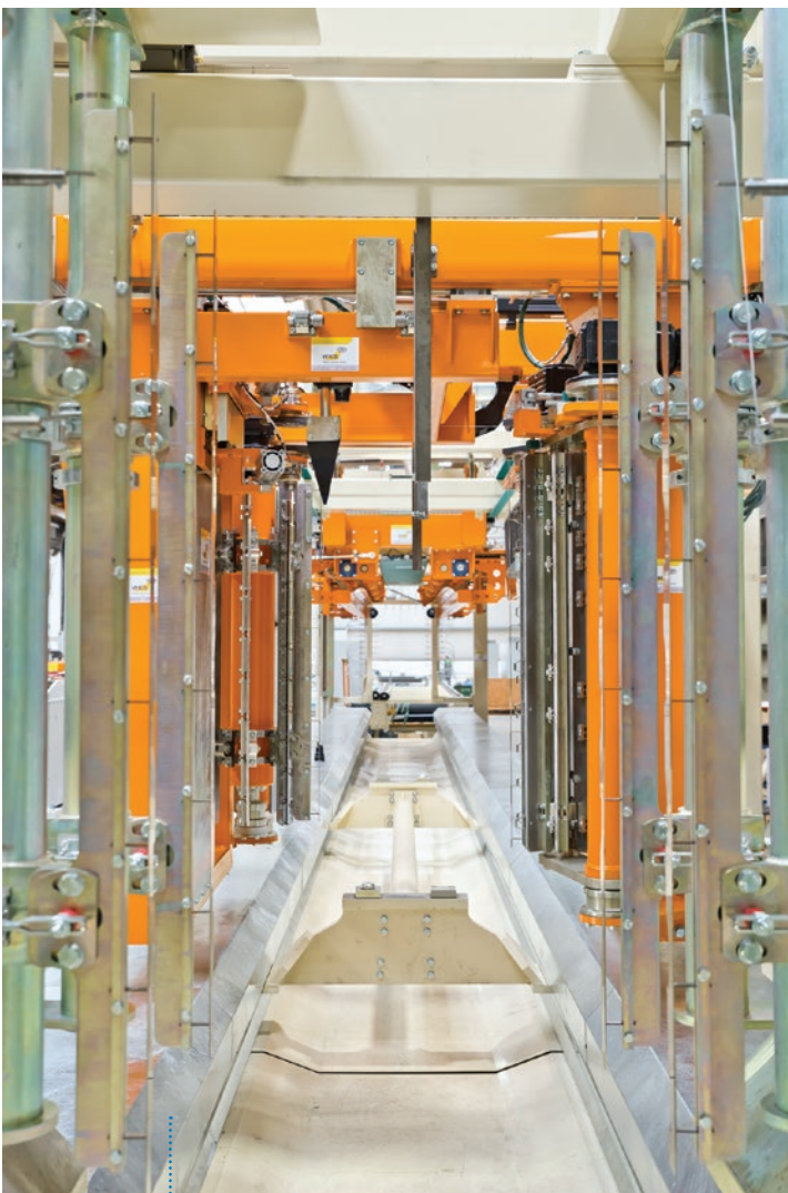
..... Cutting line for blocks/panels of 50 to 500 mm thickness.
