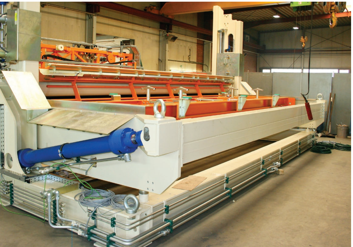
Tilting table after the cutting line to tilt the cake on a hardening grate.
